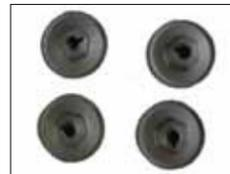
Remove four OEM nut washers and save for reuse.
