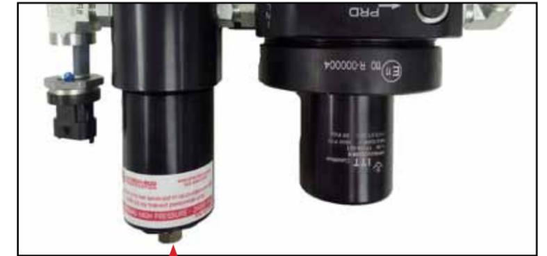
**NOTE:** For the 2018 model year, the bleeder valve plug is located on the coalescing filter.
