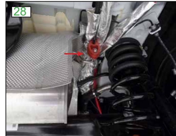
Note: For the 2018 model year CNG system, the bleeder valve is located on the coalescing filter and not on the cross assembly.
