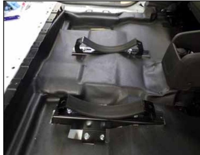
You may also modify this area of the floor mat to fit cylinder base brackets once at the bracket install step.
