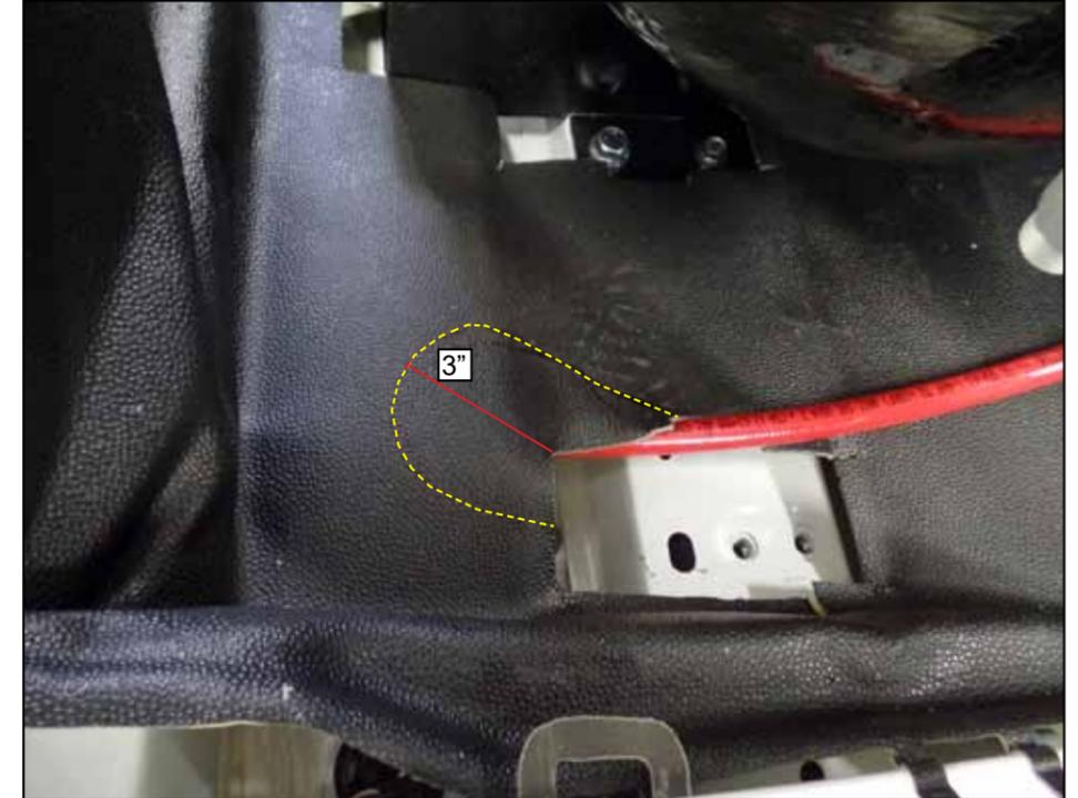
Modify mat to allow high pressure hose to run through.
